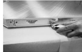
3. Drill out pop rivet at opposite end of door hinge. Use 3/16” Drill bit.
