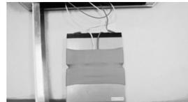
Insert battery into battery compartment with attention to wire leads collecting between battery and rear sign face. Close door and insert 3/16” aluminum rivet or sheet metal screw to secure door. Turn power “On” at key switch.
